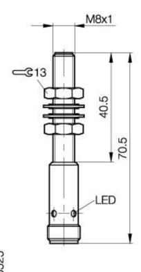
**Inductive Sensors** BES 516-527-S 4-H M8x1 x 70.5 normally-closed **Sn=1,5mm** shielded
